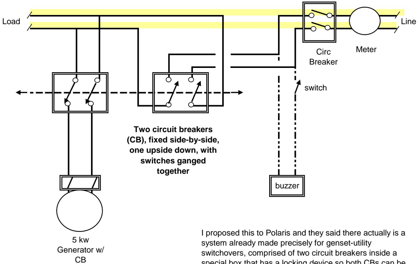
I proposed this to Polaris and they said there actually is a system already made precisely for genset-utility switchovers, comprised of two circuit breakers inside a special box that has a locking device so both CBs can be ON only alternately. But the box alone cost P4,200, and the matching CBs were about P800 each. And switchover is a more complicated procedure of 4 steps.
