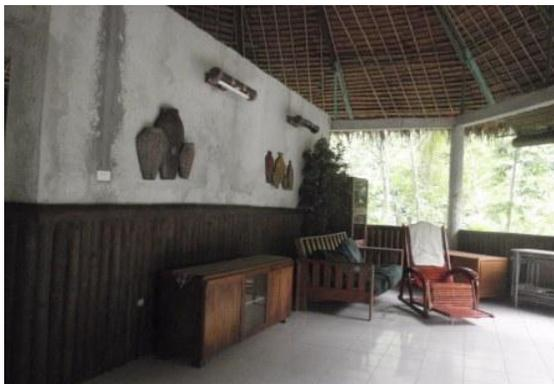
Its hexagonal base is concrete, sitting on concrete pylons that raises it up for a commanding view of the nearby river, water falls, swimming pools, as shown, (yours truly on left, and grandson on right). Walls are "sawali" bamboo woven slats; roof is "nipa" thatch tied to steel roof trusses, with concrete beam members.
