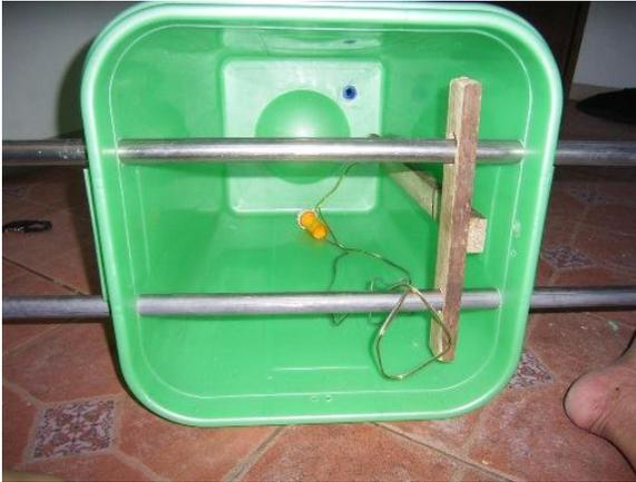
Left: The overhead tank is a plastic water container with a hole bored at the bottom for the entry/outlet pipe, with plastic garden hose fittings. The tank is hung from the eave's roof rafters using the supporting metal pipes that also locate the wooden crossbeam that holds the float switches inside the tank. Various holes drilled through the wood allow height adjustment for the switches.
