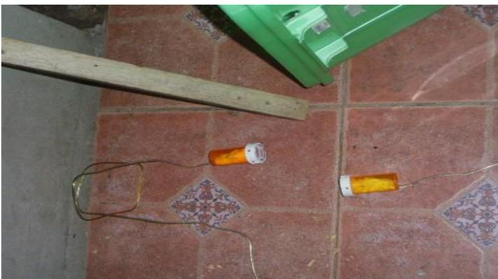
Left: The float switches which signal the pump when to start and stop are plastic medicine bottles that house mercury switches taken from an old air-con thermostat, waterproofed by epoxy. For safety, 12 volts was used for these switches, sourced from a 3 ampere boxed power supply similar to those types one can get at Radio
